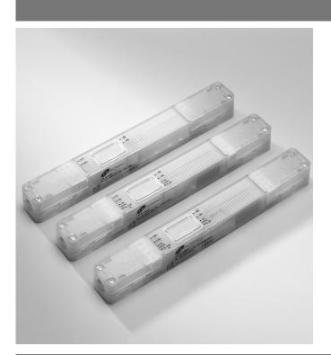
The DA-SL-AP series are a range of DALI addressers that can be setup using the UNLCDHS programming handset and the DM-ADP-PRG programming adaptor. An addresser takes in a message from an addressable DALI system and translates it into a broadcast message so that the luminaire ballast(s) does not have to be addressed using a PC or other methods.
